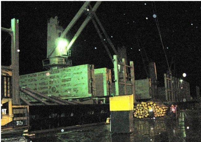
maximum capacity. The logs are loaded to 6 metres above the deck in the winter and 8 metres in the summer. In the winter logs are 6-7% heavier than in summer. To load this ship in one port it would take about 58 hours and to unload in Korea the logs will be loaded on to barges which will take 7 days. The barges take the logs closer to the mills.
